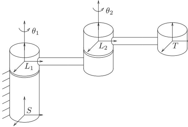
Figure 3.2: A two degree of freedom manipulator.
