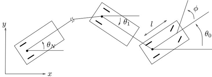
Parameterize the configuration by the states of the automobile plus the angle of each of the trailers with respect to the horizontal. Show that the control equation for the system has the form
