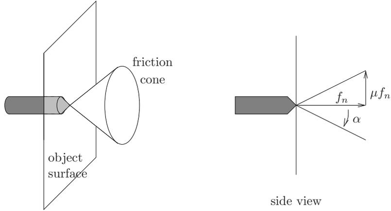
Figure 5.4: Geometric interpretation of the Coulomb friction model.
