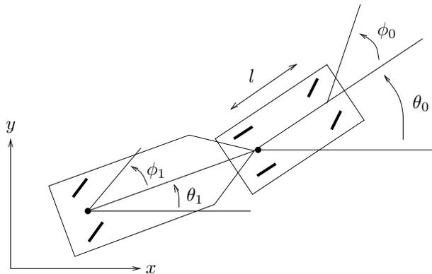
The constraints on the system are similar to that of the car in Section 3, with the difference that back wheels are steerable. Derive the nonlinear control system for a firetruck corresponding to the control inputs for driving the cab and steering both the cab and the trailer, and show that it represents a controllable system.
