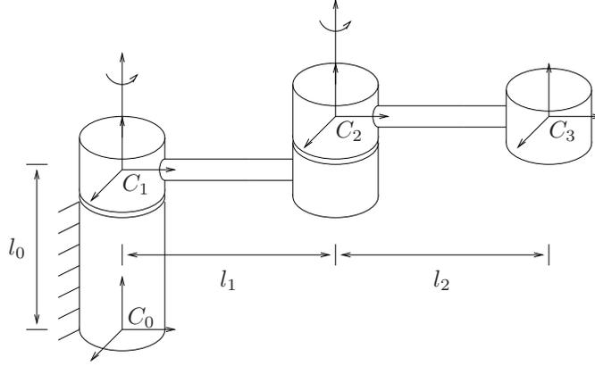
Figure 2.17: A two degree of freedom manipulator.
