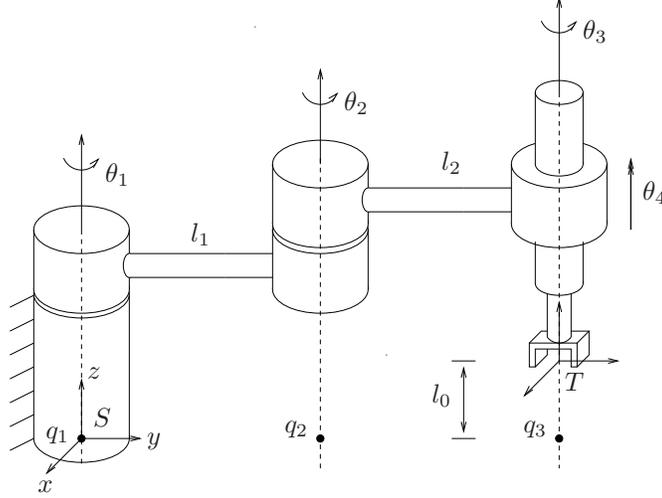
Figure 3.12: SCARA manipulator in its reference configuration.
