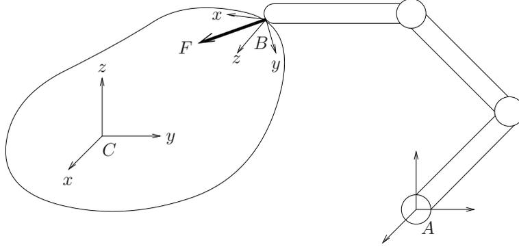
Figure 2.13: Transformation of wrenches between coordinate frames.
